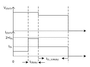
Figure 7-1. Timing Waveforms
