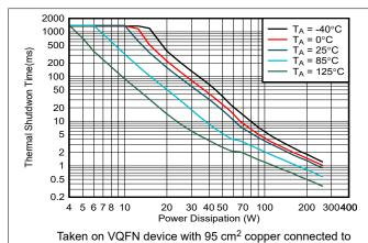
Figure 6-7. Thermal Shutdown Time vs Power Dissipation for RGE Package
