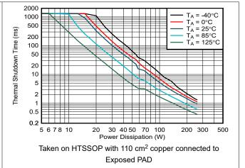
Figure 6-8. Thermal Shutdown Time vs Power Dissipation for PWP Package
