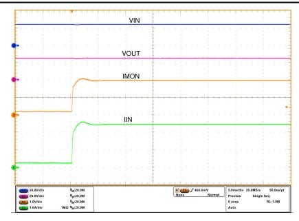
Figure 8-7. IMON Response During a Load Step
