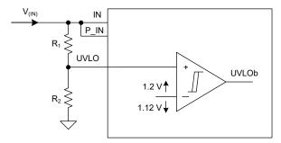
Figure 8-3. UVLO Thresholds Set by R<sub>1</sub> and R<sub>2</sub>
