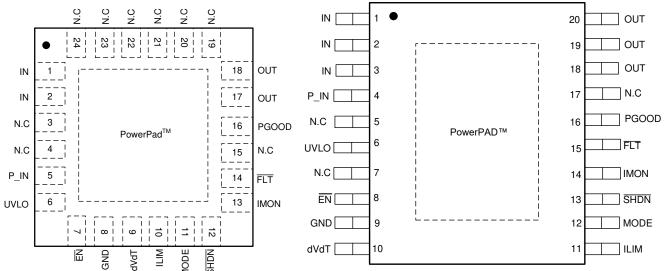
Figure 5-1. TPS16530 RGE Package 24-Pin VQFN Top View
