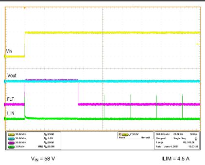
Figure 8-6. Start-Up With Short on Output
