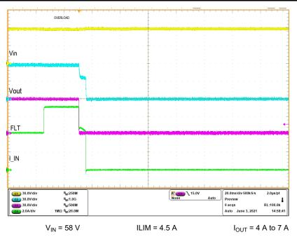
Figure 8-4. Pulse Current Support
