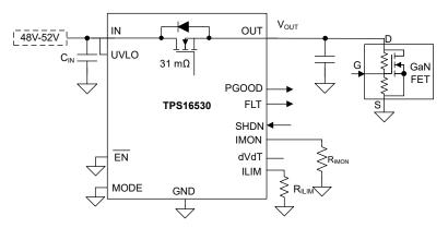
Figure 9-8. TPS16530 Configured for 48-V Power Amplifier Protection
