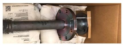
Image 1 (above) depicts a sampling probe where the customer was concerned about inaccurate measurement of sulfides in the collected samples. It was believed that the skewed measurements originated from cross-contamination of sulfide leaching into the metallic sample cylinder and system components. A SilcoNert 2000 coating was applied to the probe, providing an inert and corrosion resistant barrier that will prevent any metal ion leaching or contamination of the sulfide readings.
