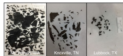
Figure 3. Samples of starch based biodegradable plastic mulch (BioTELO ® ) recovered after twenty four months burial in the field at three experimental locations. Photo credit: J. Moore-Kucera, Texas Tech University.
