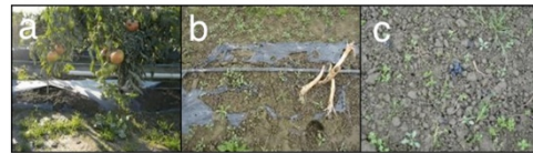
Figure 2. (a) Starch-based biodegradable plastic mulch (BioAgri ® ) in experimental field plots during harvest, 135 days after laying mulch. (b) 9 months post-harvest on soil surface, 348 days after laying mulch. (c) 9 months post incorporation, 348 days after laying mulch. Photo Credits: J. Cowan (2a) and C. Miles (2a, 2b), Washington State University. From Corbin et al., 2013.
