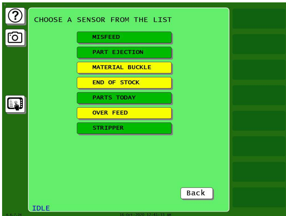
Figure 13- The list of previously programmed sensors from which the timing and stop type settings can be copied to the new sensor
