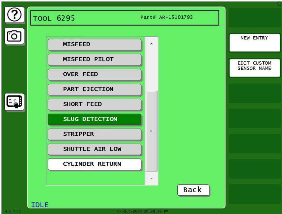
Figure 1- The sensor name screen showing the reduced list of canned names and the NEW ENTRY button for creating a custom sensor name
