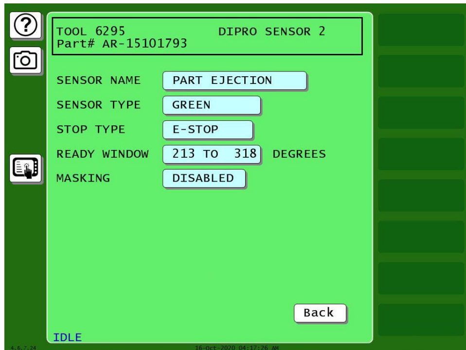
Figure 8- Sensor Summary Screen showing the Masking feature disabled. This is the default setting.
