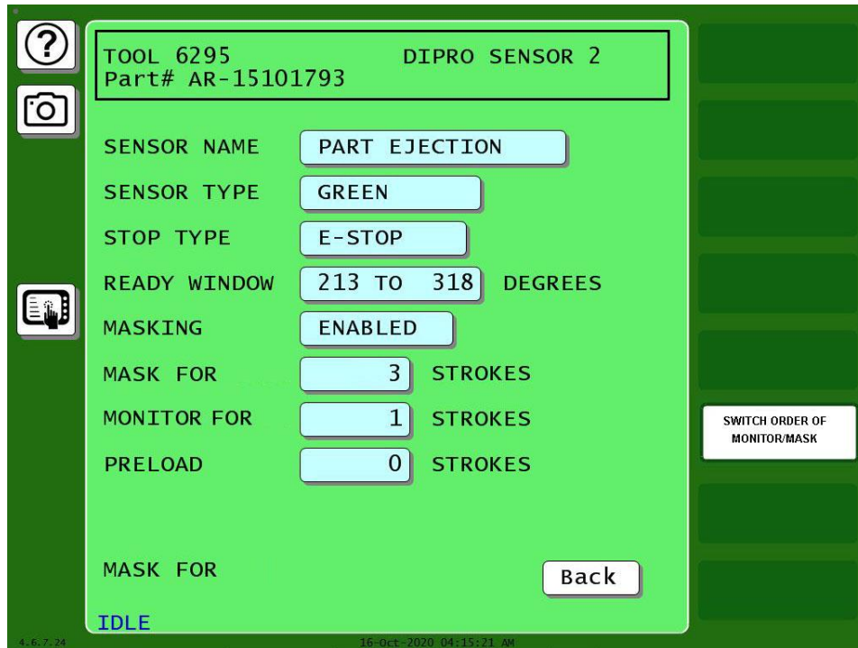
Figure 9- Standard Green sensor type with masking enabled. This sensor will check for part ejection every 4th stroke
