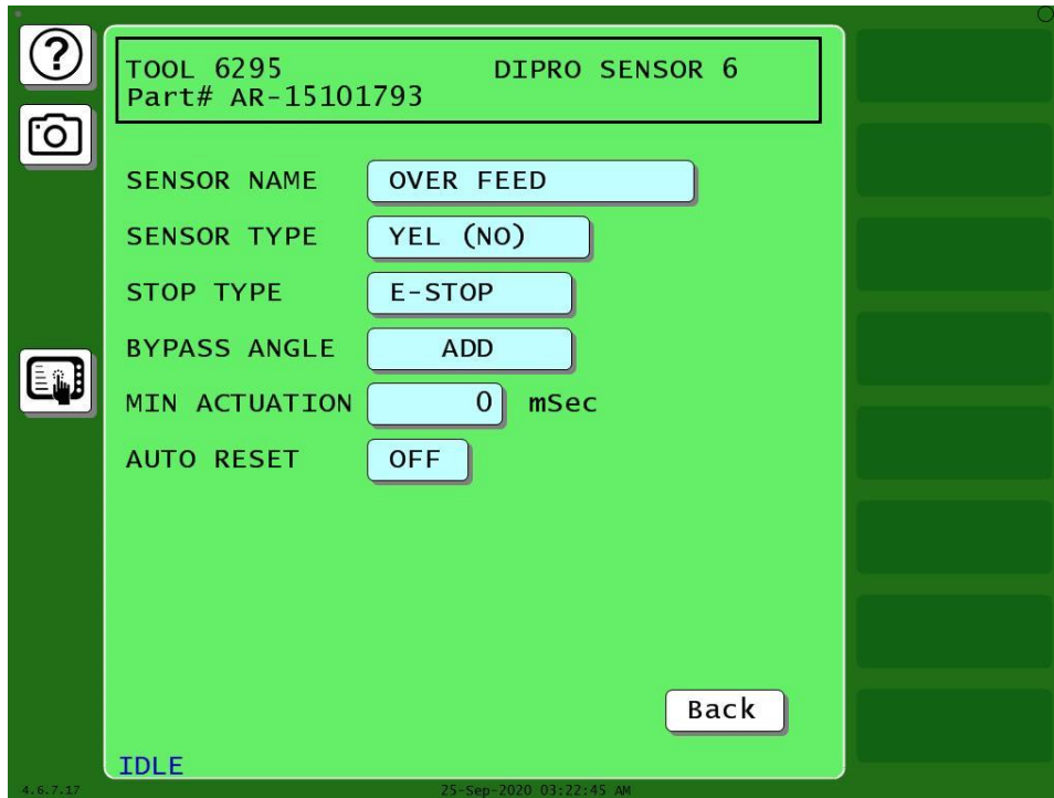
Figure 6- The sensor programming summary screen for a Yellow sensor showing the bypass, minimum actuation time, and auto reset settings
