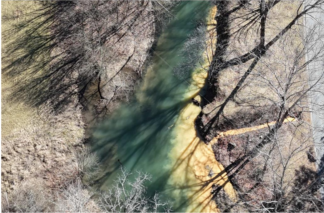
Figure 4 - a spring contaminated by upslope MVP work carrying heavy sediment loads to Sinking Creek, January 31, 2024.
